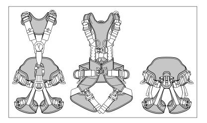
$\bullet$  Check the condition of the elastic and/or plastic keepers (cuts, wear, tears...).
