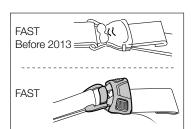
• Check that the straps are correctly threaded, with no twists.
