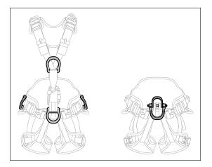
• Check the condition of the textile attachment points (cuts, wear, tears...).
