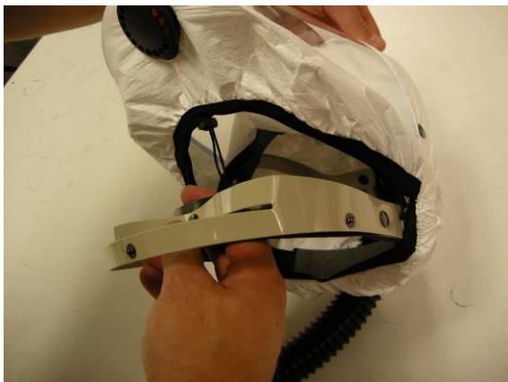
Lift the head harness out of the hood and withdraw the hose.
