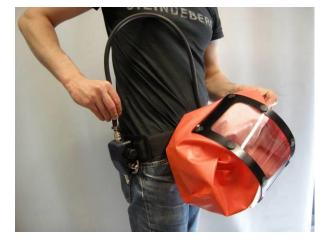
• Connect the breathing hose of the hood to the outlet of the control valve.
