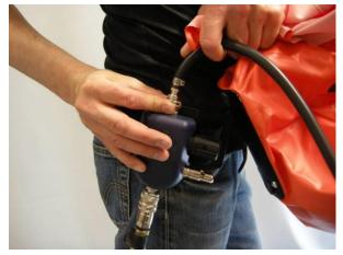
Releasing the compressed air tube / breathing hose Both couplings are of safety type and are released in two stages.
