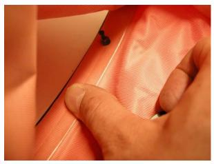
• Press the visor towards the frame all round, so that the tape will stick to the hood material.
