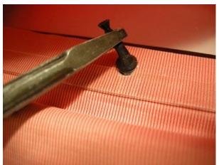
• Fit the visor, with the tape facing downwards, over the rubber studs. Bear in mind that the holes for the head harness screws must be oriented in the same direction as the hood and frame. Secure with the studs, possibly using a pair of pliers.
