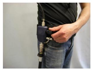
• Use the control valve knob to set the air flow rate to suit the work intensity. In the fully closed position (turn anticlockwise), the flow is around 150 l/min, while in the fully open position (turn clockwise), it is around 240 l/min.
