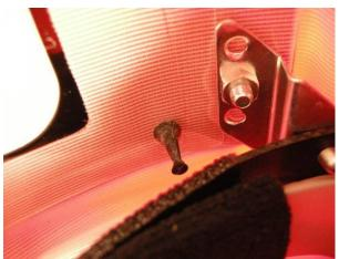
• Fit the head harness. Make sure that the beads in the mounting plate of the head harness are oriented into the guide holes in the visor. Finally, check that the work has been correctly done.
