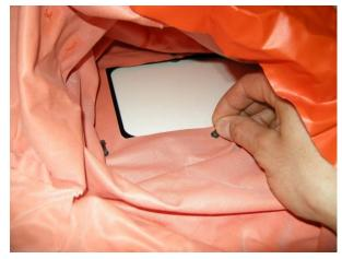
• Place the hood over the frame and insert the 4 studs into the corresponding holes in the hood.
