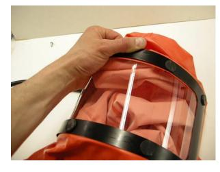
• Bend the frame to the required shape. Align the vacant holes for the studs in the frame, hood and visor. Insert the studs and secure them by pulling the studs from the inside of the hood. The simplest procedure is to fit one stud at a time.
