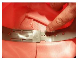
To adjust the height The head strap of the head harness consists of two halves. The upper half runs in a groove in the lower half. The position is determined by means of a pin in the lower half that engages in one of the holes in the upper half.
