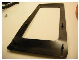
• Straighten the frame or fit a new frame, and place it on a flat surface with the short side towards you. Fit 4 studs into the two furthest holes on each side.
