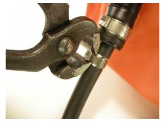
• Release the hose from the hood by cutting off the hose clip with a pair of nippers.
