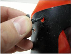
• Pull off the 8 rubber studs, and remove the frame and visor.
