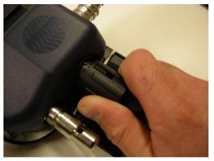
• Turn the control valve knob anticlockwise as far as it will go, in order to throttle the air flow rate to a minimum.
