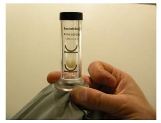
• Grip the flow meter with the other hand and hold it so that it points vertically up from the bag.
