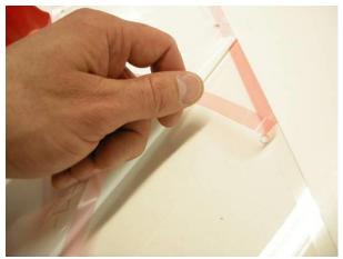
• Remove the protective films from the visor and from the double-sided adhesive tape.
